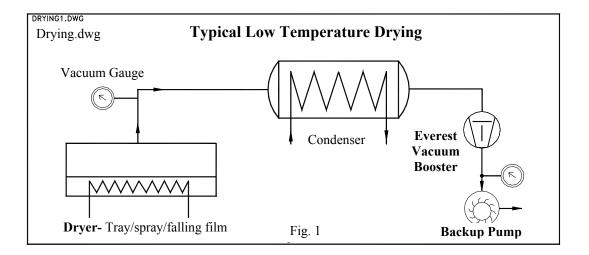
A vacuum Booster, when used in conjunction with any of the above, over comes all the associated limitations and increases the overall process efficiency by increasing the vacuum and pumping speeds with relatively very little extra energy.
