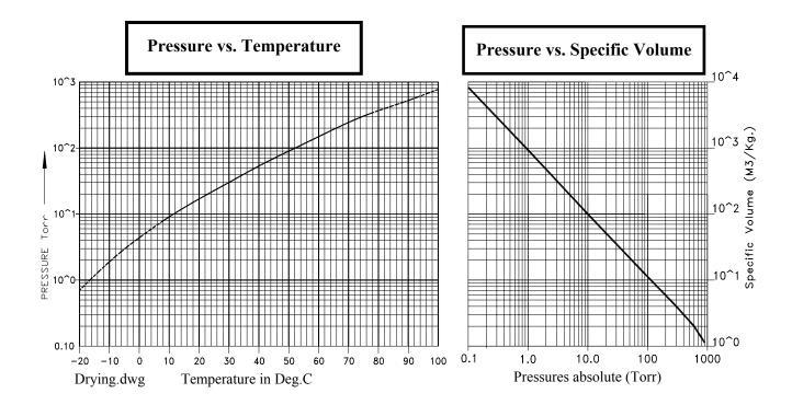
From the above graph we see that at about 4 Torr, it is possible to "boil the water" at 0 degrees C. Accordingly Drying can take place at low temperatures, to meet the process requirements, provided the corresponding suitable pressures are maintained.
