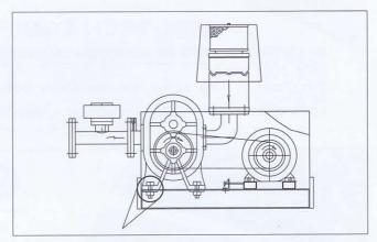
Soft foot: When anchoring a unit down, any contact point between the feet and the mounting must be shimmed to be sure the blower feet are square with the base. Do not tighten the bolts to solve a soft foot condition without shimming.
