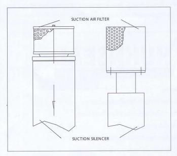
Clean Air Filter every fortnight by reverse air flow. Chocked filter would result in excessive power consumption and overheating of the blower. Replace filter every three months or earlier, if inspection so demands. Check and clean Air Silencer every month.
