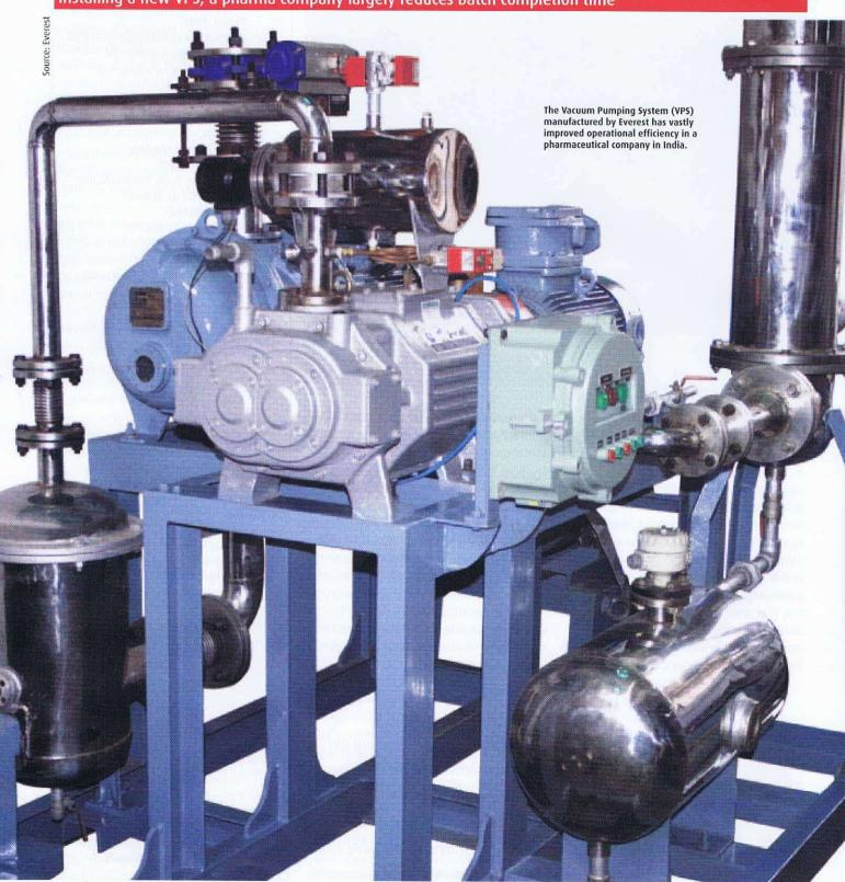
As a replacement of the existing steam jet ejector at M/s XYZ Pharma Ltd. (name changed to keep the user's identity secret), Everest Blower Systems has recently installed a Vacuum Pumping System (VPS), which was manufactured in their (Everest's) factory. Here is an exhaustive case study based on the step by step commissioning report and onsite experience.
