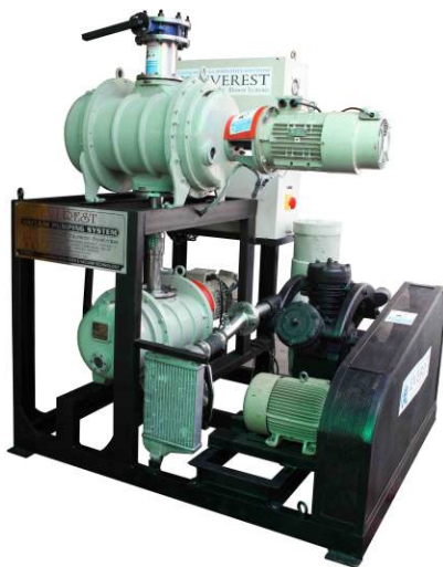
Fig: Mechanical Vacuum Booster with External Bypass Valve for regulating differential Pressure across the Booster
