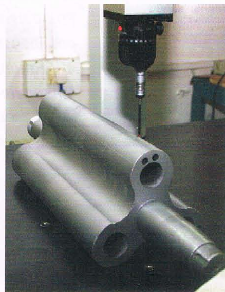
Trilobe blower rotor being checked on a coordinate measuring machine
