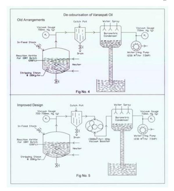
To get the required product quality higher vacuums to the level of 740 mm Hg were essential against the levels of 680-700 achieved. The available option was to install a steam ejector for which additional Boiler & accessories were also required since additional steam to the tune of 250-300 KG/hr was required. Also additional steam would add to the condenser loading and hence need for bigger condenser, demanding heavy capital investment.
