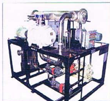
A typical vacuum pumping system designed for drying in a pharmaceutical industry
