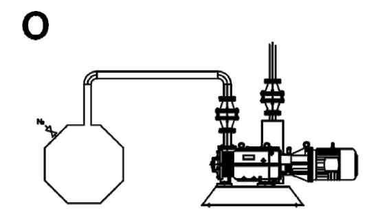
Where flammable mixtures are pumped, either Inert the system prior to evacuating or adopt flame arresters to the pump inlet and exhaust. If air is used for the seal purge, a flame arrester should be fitted to the seal purge line.
