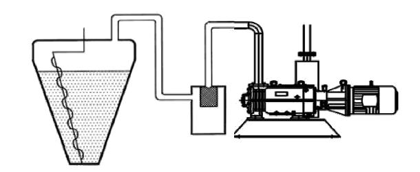
• Fit a suitable filter in front of the pump where high particulate carry over is expected (e.g.  $20\mu$ m)
