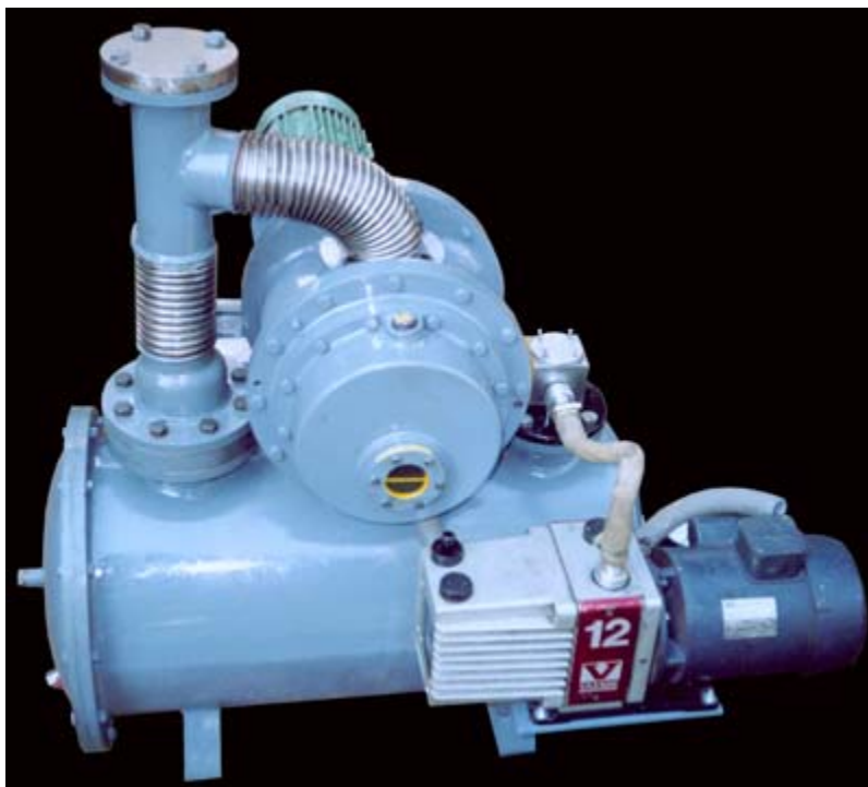
Fig: Mechanical Vacuum Booster with post condenser backed by Rotary Oil Pump for Molecular Distillation.
