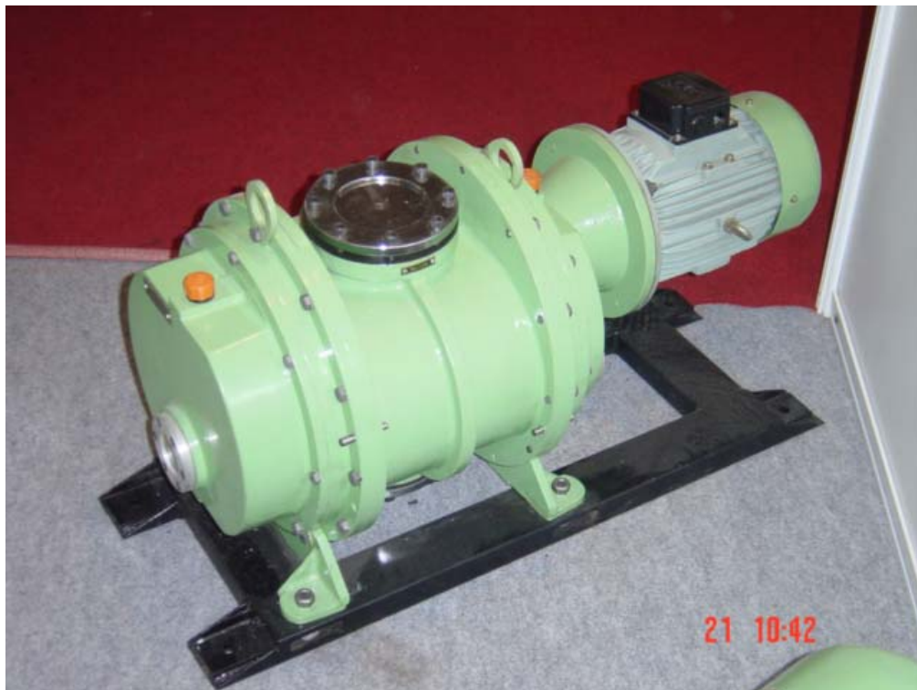
Fig: Typical Direct Mounted Mechanical Vacuum Booster Assembly
