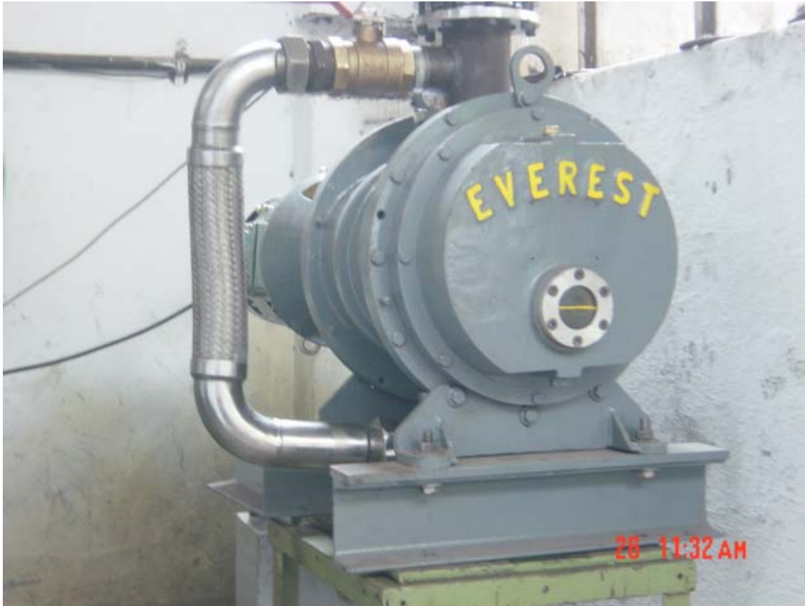
Fig: Mechanical Vacuum Booster with External Bypass Valve for regulating differential Pressure across the Booster
