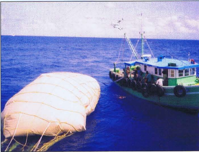
Geo Bags being used to tow fresh drinking water produced on the plant
