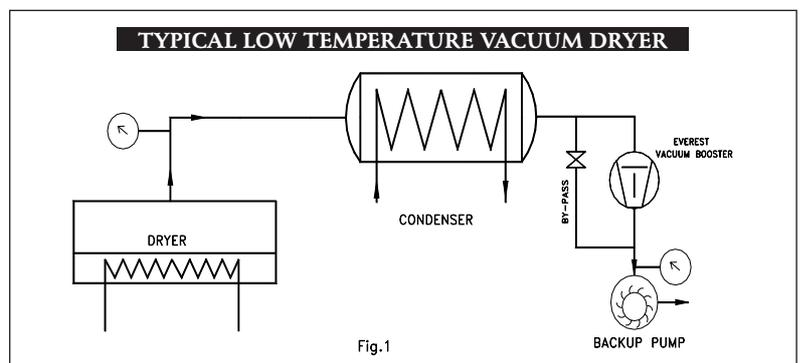
A vacuum Booster, when used in conjunction with any of the above, over comes all the associated limitations and increases the overall process efficiency by increasing the vacuum and pumping speeds with relatively very little extra energy.
