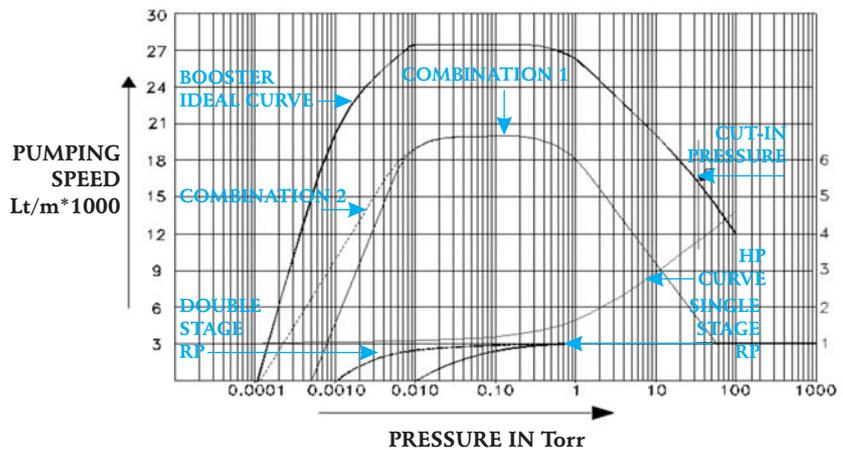
**Combination 1** Everest Booster EVB30 backed by 3000 LPM rotary pump single stage
