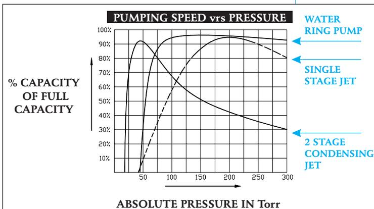
For example, a pump is to be selected to handle 10Kg/hr of air load and 5 kg/hr of water vapor load at 50°C and the process vacuum is to be maintained at 20 Torr. The pump capacity comes to
