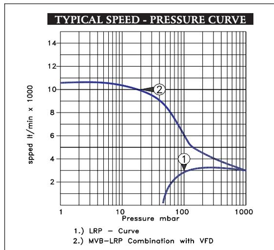
Above is a typical water ring pump speed curve. The pumping speed is equal to the rated speed (displacement) during initial pumping and thereafter drops rapidly reaching to zero at its ultimate (690 720 mm Hg). In most of the chemical processes the process vacuum is in the range of 680-700mmHg where the pumping speed of WRP is merely 15-20% of its full rated capacity. This demands installation of much larger
