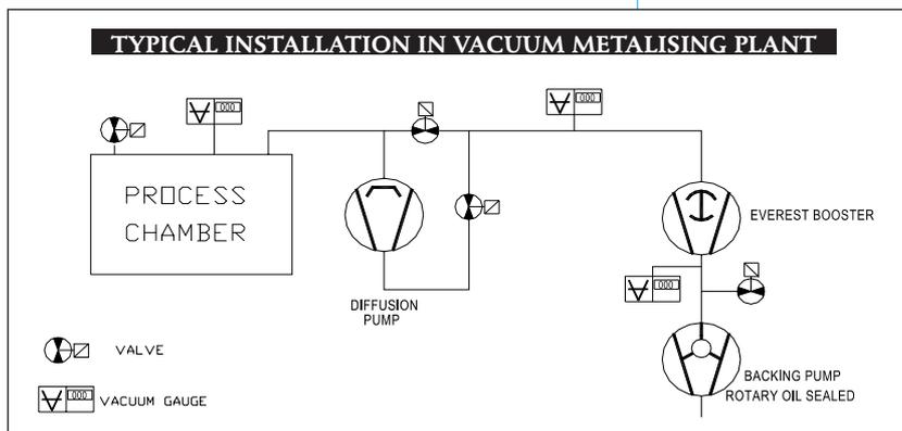
Typical arrangement of Booster installations are shown. The booster can be directly mounted on the suction of the fore pump or mounted on a base frame with connection to fore pump. For applications involving pumping of CONDENSABLE VAPOR like in distillation, a suitable condenser can be installed in between the Booster & Fore pump. In such cases the Fore pump size can be reduced drastically, to match the NON-CONDENSABLE load.
