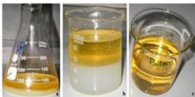
Fig. (a) Raw biodiesel and glycerin (b) Washing of biodiesel (c) Pure palm Biodiesel.
