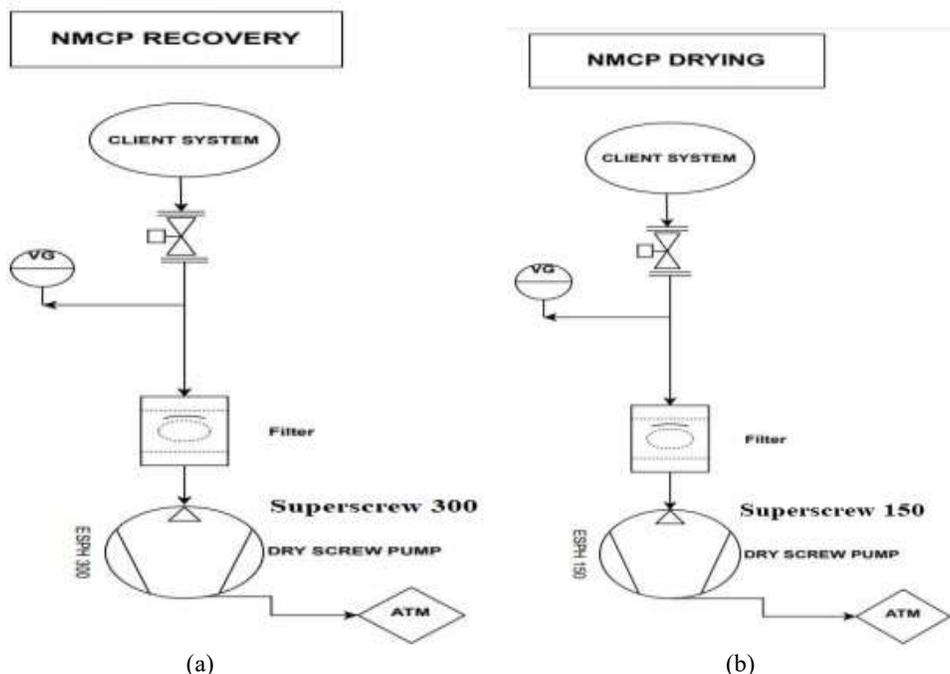
Fig 2: (a) Distillation & (b) Drying operation of N Methyl 4 ChloroPiperidine using Dry Screw Vacuum Pump
