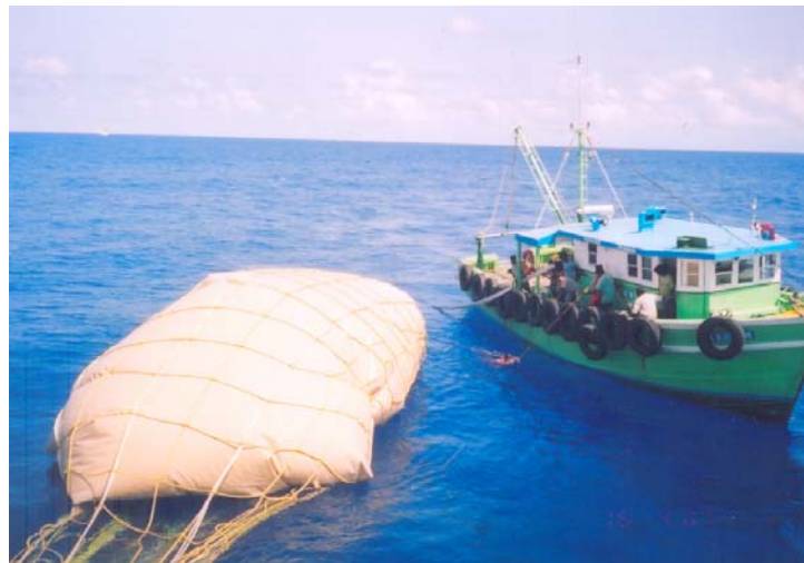
Fig 18 & 19: Geo Bags being used to tow fresh drinking water produced on the World's First Floating Barge Mounted Low Temperature Thermal Desalination Plant to shore
